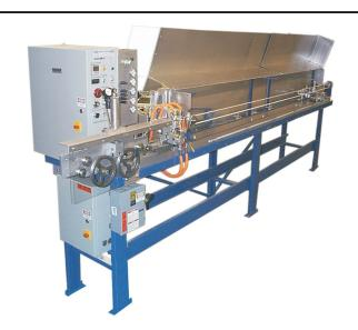
Custom designed automatic machines for cutting to length and fusing the ends of stranded cable in most metals.
