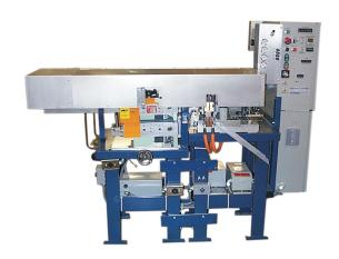
Custom designed machines for cutting to length and fusing the ends of stranded cable in most metals, flexible drive shaft or stainless steel overbraided Teflon hose.
